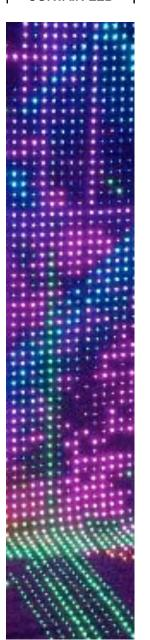
There are 24x100 = 2400 leds in the curtain, you need to set up Width: 192 and Height: 100. Since you are going to directly control the led curtain with computer, select "Network Adapter. Click OK.
